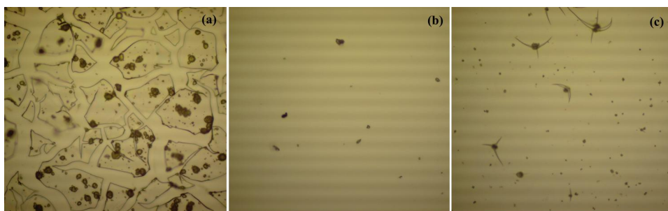
Figure 1. Optical microscopy images of (a) SiO 2 /PEG/TiO 2 , (b) SiO 2 /PEG/ZnO and (c) SiO 2 /PEG/TiO 2 /ZnO films.
