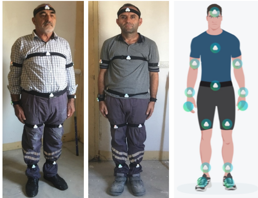
Figure 7. Placement of 11 IMU sensors on the construction workers.
