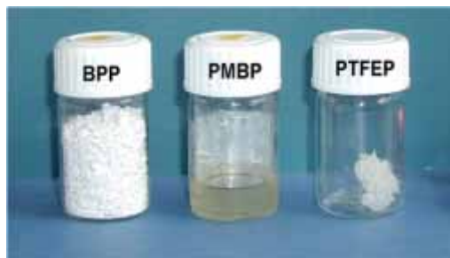
Scheme 6. Illustration of the variable physico-chemical properties of polyphosphazenes by changing or mixing the substituents [18,19]; the three polymer samples have average molecular weights around 10^5 g/mol.
