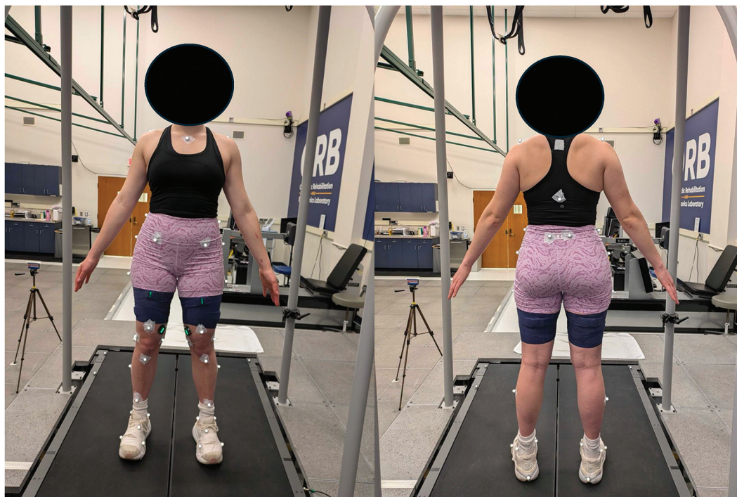
Figure 1. Retroreflective marker placement. The left photograph shows the anterior view, and the right photograph shows the posterior view.
