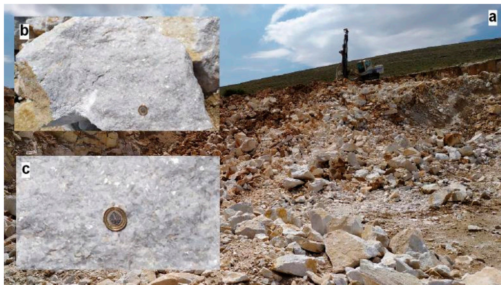
Figure 6. Field (a) and close-up (The 1 Turkish lira coin was used as the scale) (b,c) views of white marble (BC-4), south of Alişar.
