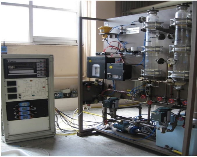
Fig. 2 Process control simulator developed with wireless control purpose
