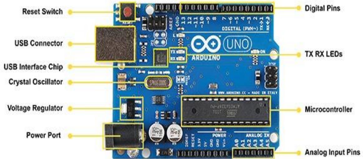
Figure 3.3. Components of Arduino UNO Board
