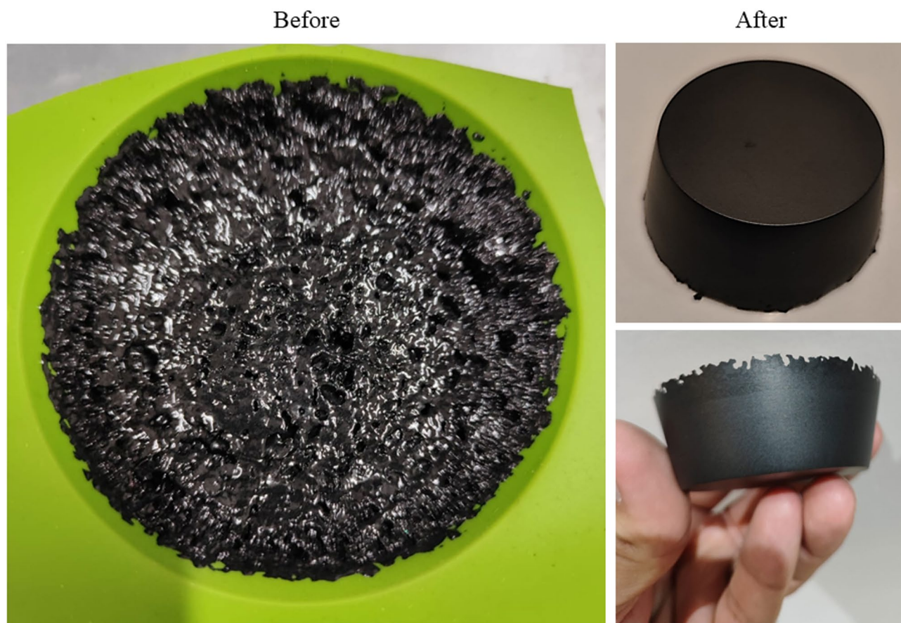
Fig. 13. Schematic illustration of the neutron shielding fabrication process before and after curing.
