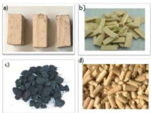
Figure 3. Feedstocks a) Pine blocks, b) Fir blocks, c) Lignite, and d) Pellets
