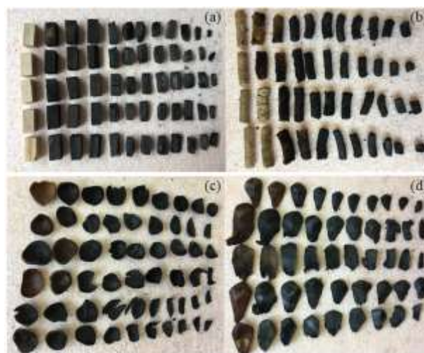
Figure 4. Size evolution of solid blocks in the gasification process a) pine block b) pellet c) hazelnut shell d) pinecone
