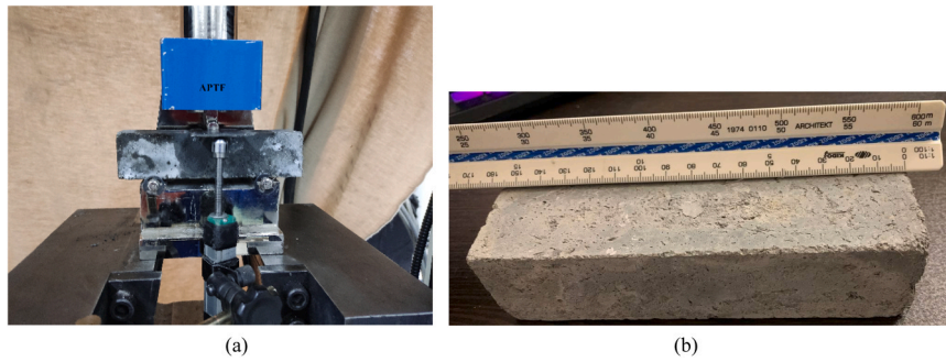
Fig. 6. (a) Flexural strength test specimen; (b) three-point bending test setup.
