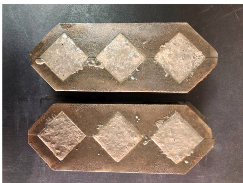
Fig. 5. Specimens used for the compressive strength experiment.
