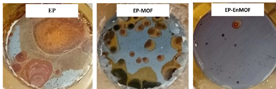
Figure 16. Visual images of the EP, EP-MOF, and EP-EnMOF coatings upon completion of the corrosion tests.
