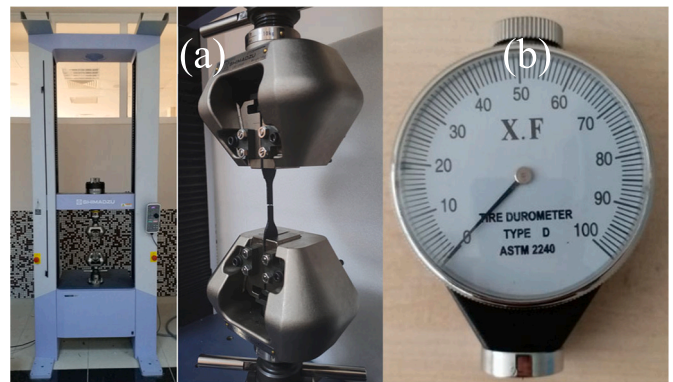
Fig. 1. (a) Shimadzu AGS-X universal testing machine and (b) X.F Shore D hardness tester.
