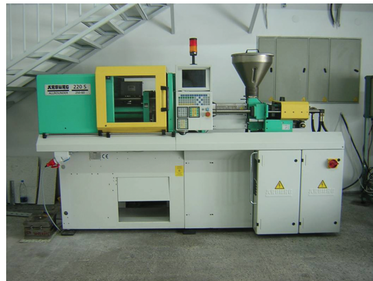
Fig. 7. Arburg all-rounder 220 s injection molding machine.
