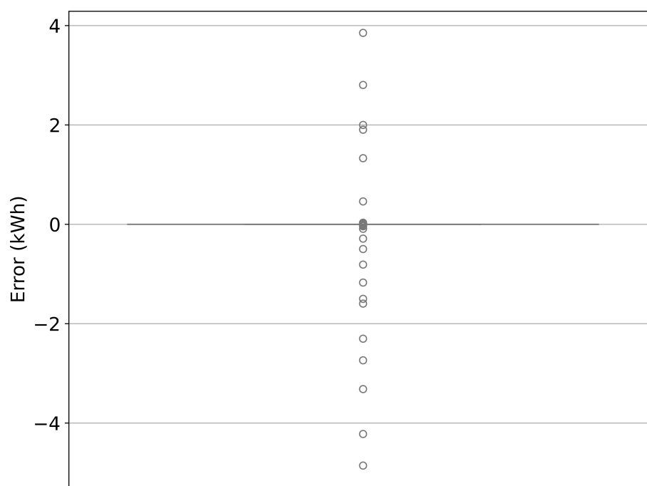
Figure 6. Distribution of forecasting errors showing the majority of predictions within \pm 1 kWh of actual values, with a few outliers.
