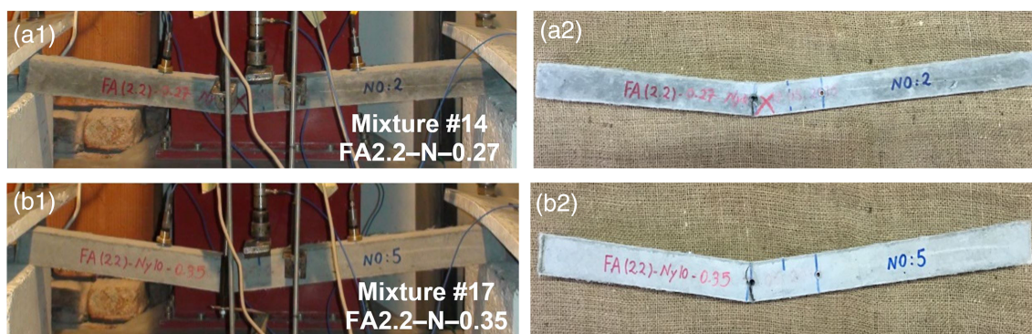
FIGURE 8 Representative photos showing the effect of W/B ratio on impact response of ECC
