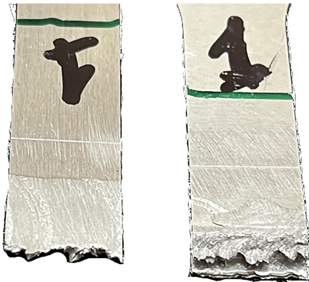
Fig. 18 Fracture region of a specimen after tensile testing
