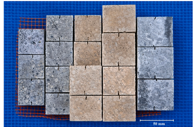
Fig. 3. Specimen preparation and setup for exposure to the aggressive environment.
