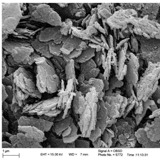
Fig. 2. Scanning electron microscopy (SEM) micrograph of the LDH nanoparticles.
