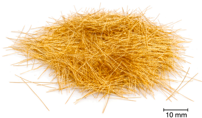
Fig. 1. The brass-coated steel microfibers employed in this study.
