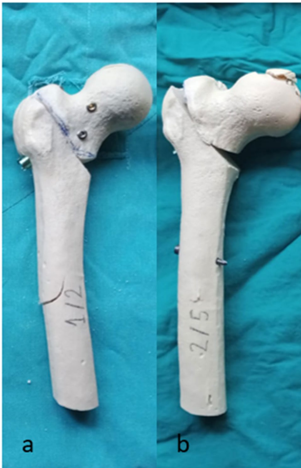
Fig. 6 Failure types after load to failure test. a The fracture occurred around to distal locking screw at the poller screw applied group. b Lag screw cut-out due to advanced varus collapse in the control group
