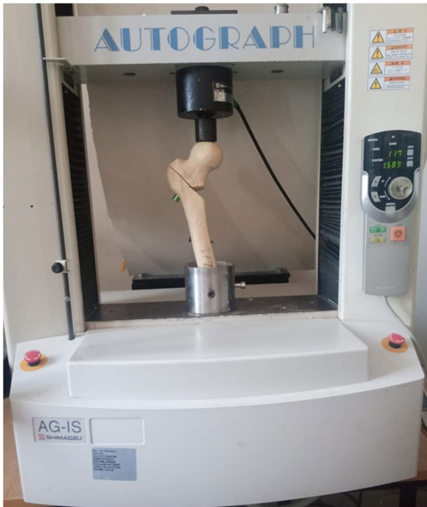
Fig. 3 Biomechanical testing setup. The specimen is mounted in a 10 cm custom metal cylinder with a 25° adduction at the coronal and 10° posterior flexion at the sagittal plane
