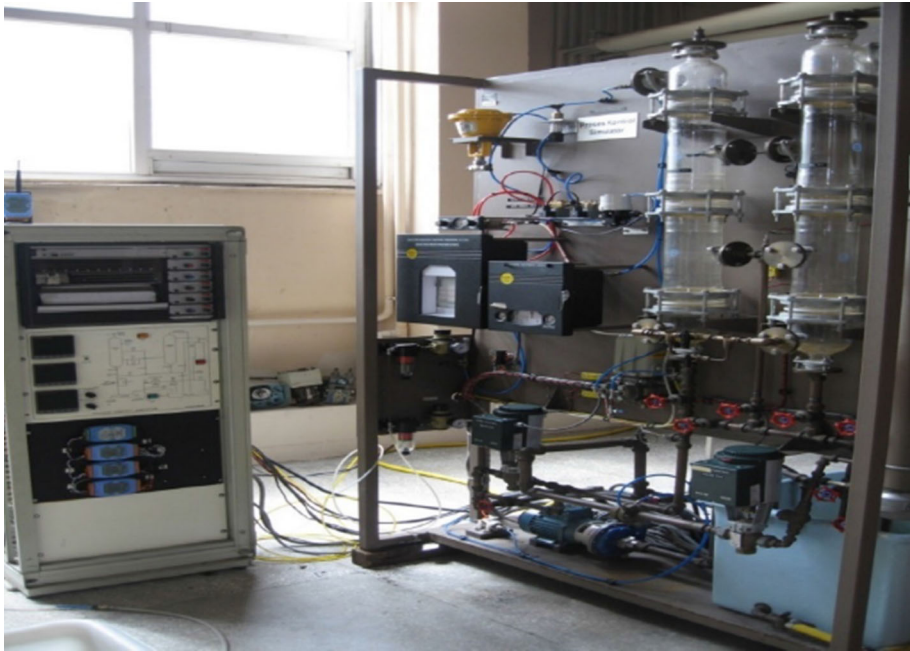
Fig. 1 Process control simulator modified for distributed wireless control purpose
