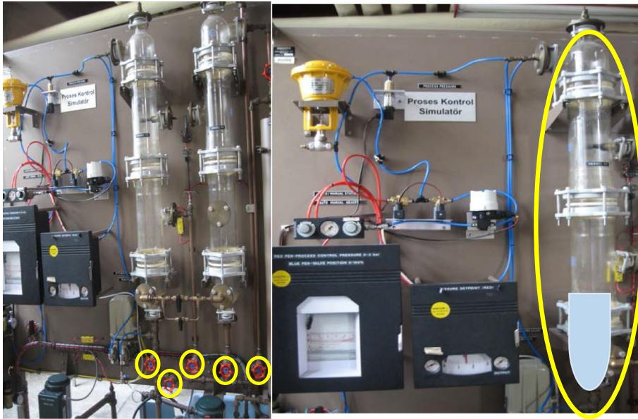
Fig. 2 V2 tank in the liquid level system and manually adjustable flow rate valves
