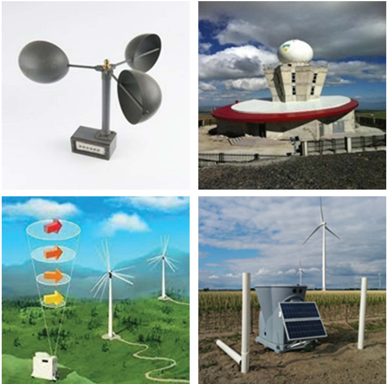
Fig 2. a) Anemometer [12] b) TDWR [13] c) LIDAR d) SODAR [14].
