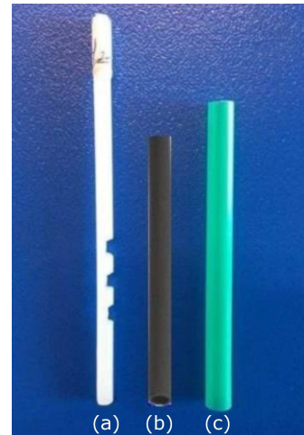
Fig. 2. From left to right, (a) PVC, (b) heat shrink tube and (c) polyurethane material of one TLD stick.
