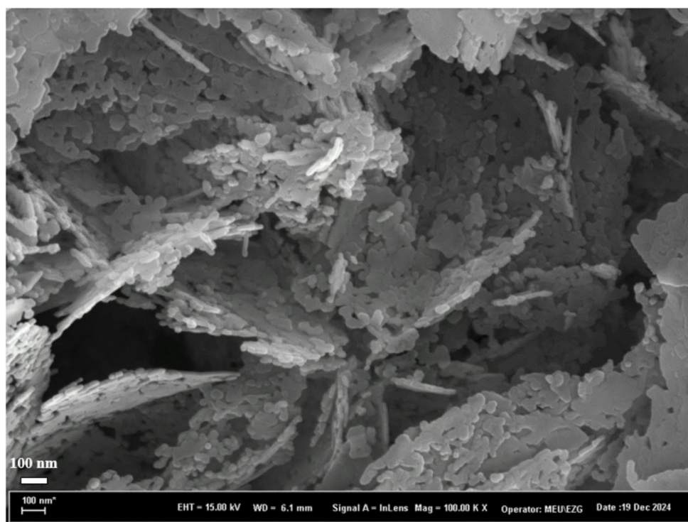
Fig. 5 FE-SEM images of NiO nanoparticles and the corresponding FESEM-based particle size distribution histogram with Gaussian fitting
