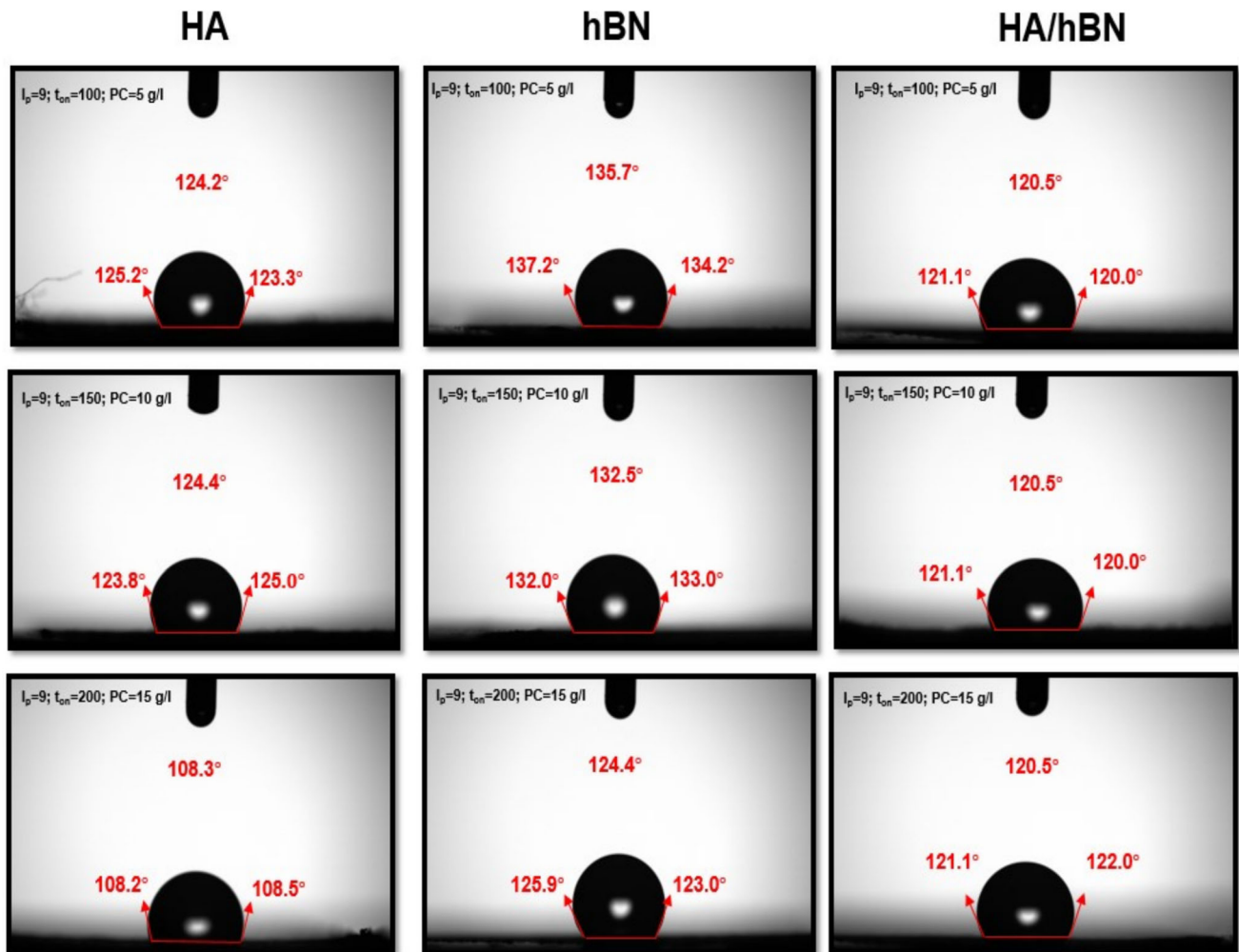
Figure 5. Static water contact angle measurements for Ti6Al4V samples processed with PMEDM using HA, hBN, and HA/hBN powder additives at various concentrations, illustrating variations in surface wettability and hydrophobicity depending on powder type and process parameters.
