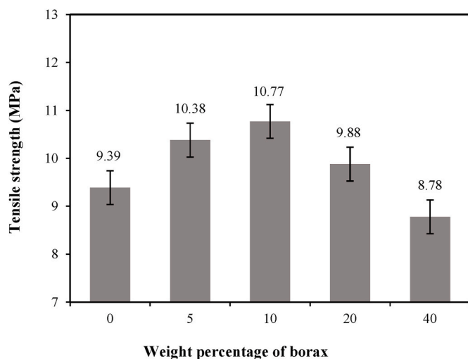
Fig. 4. Variation of tensile strength of pure polyester and composite samples with weight percentage of borax.
