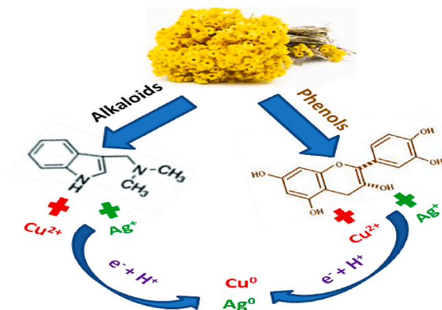
Fig. 2. A possible mechanism for green synthesis of Cu NPs and Ag NPs from Helichrysum arenarium plant extract. (For interpretation of the references to colour in this figure legend, the reader is referred to the Web version of this article.)
