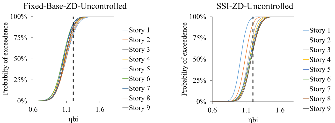
Fig. 12. Fragility curves for torsional irregularity on ZD soils (FB vs SSI).
