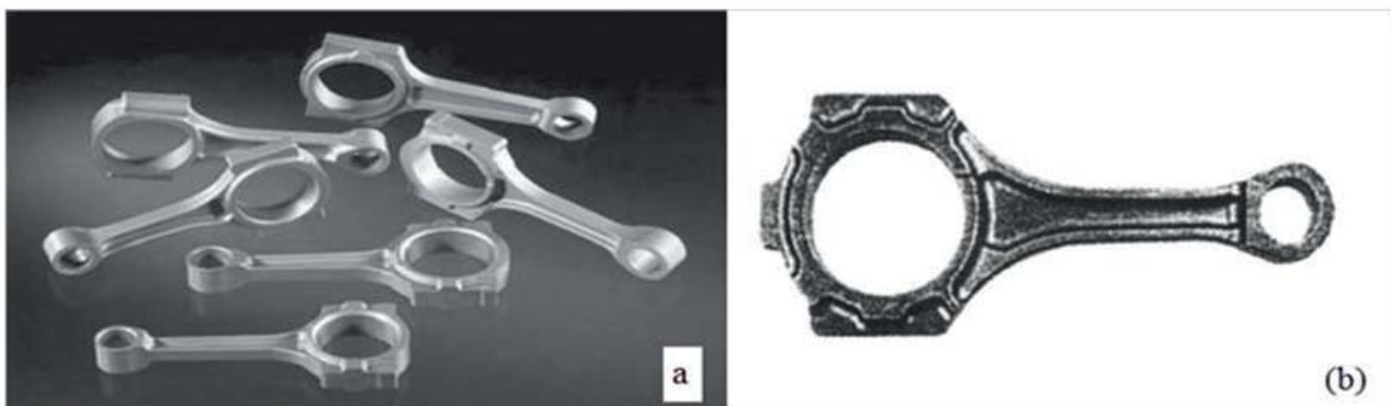
Figure 11. PSM-produced rod: a) production of GKN company, b) production of Toyota engine
