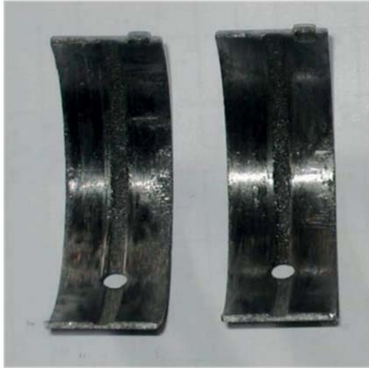
Figure 22. Crankshaft master bearings coated by FSM using a new alloy of Pb, Sn, Cu and ZrO 2 powders
