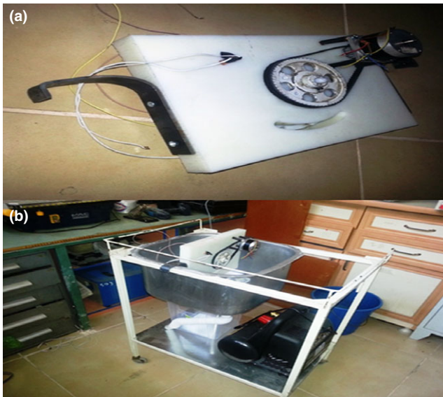
FIGURE 3 (a) Disk system in which the eggs are poured. (b) The skeleton of the device as an unmounted structure [Colour figure can be viewed at wileyonlinelibrary.com ]
