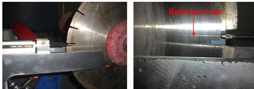
Fig. 15 Wear measurement system and reference point on the saw
