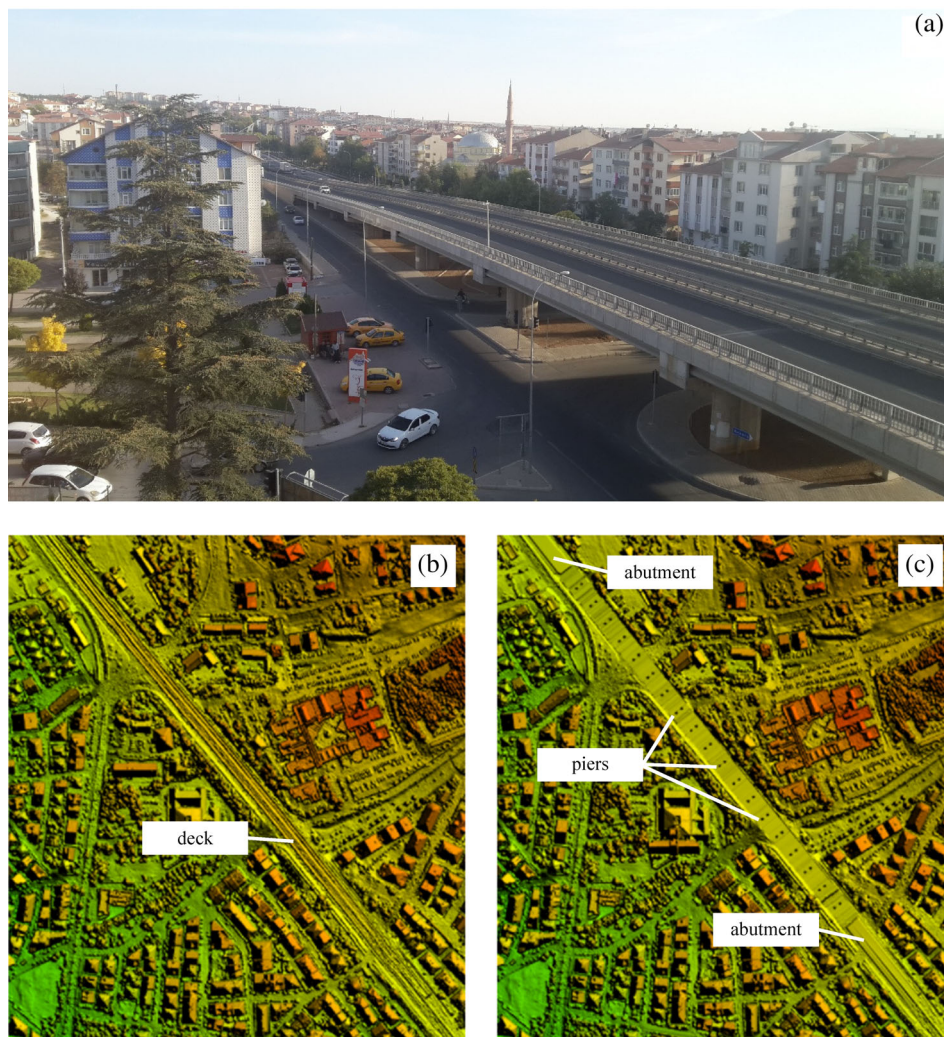
FIGURE 4 An example for DSM modifications (a) Hastane overpass on the D260 road; (b) unmodified DSM section; (c) modified DSM section
