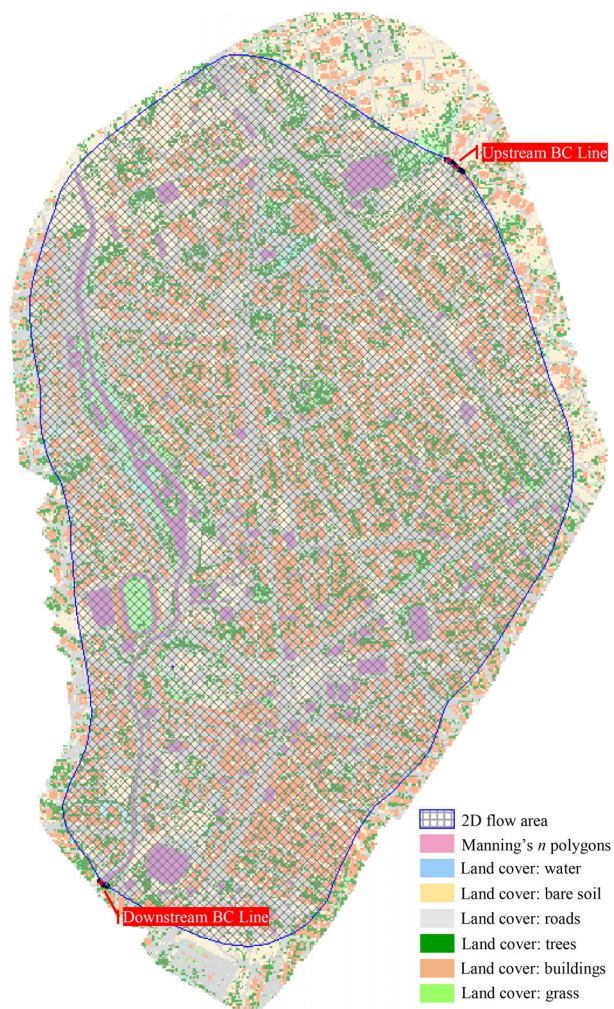
FIGURE 5 Geometric data representation in HEC-RAS 5.0 software
