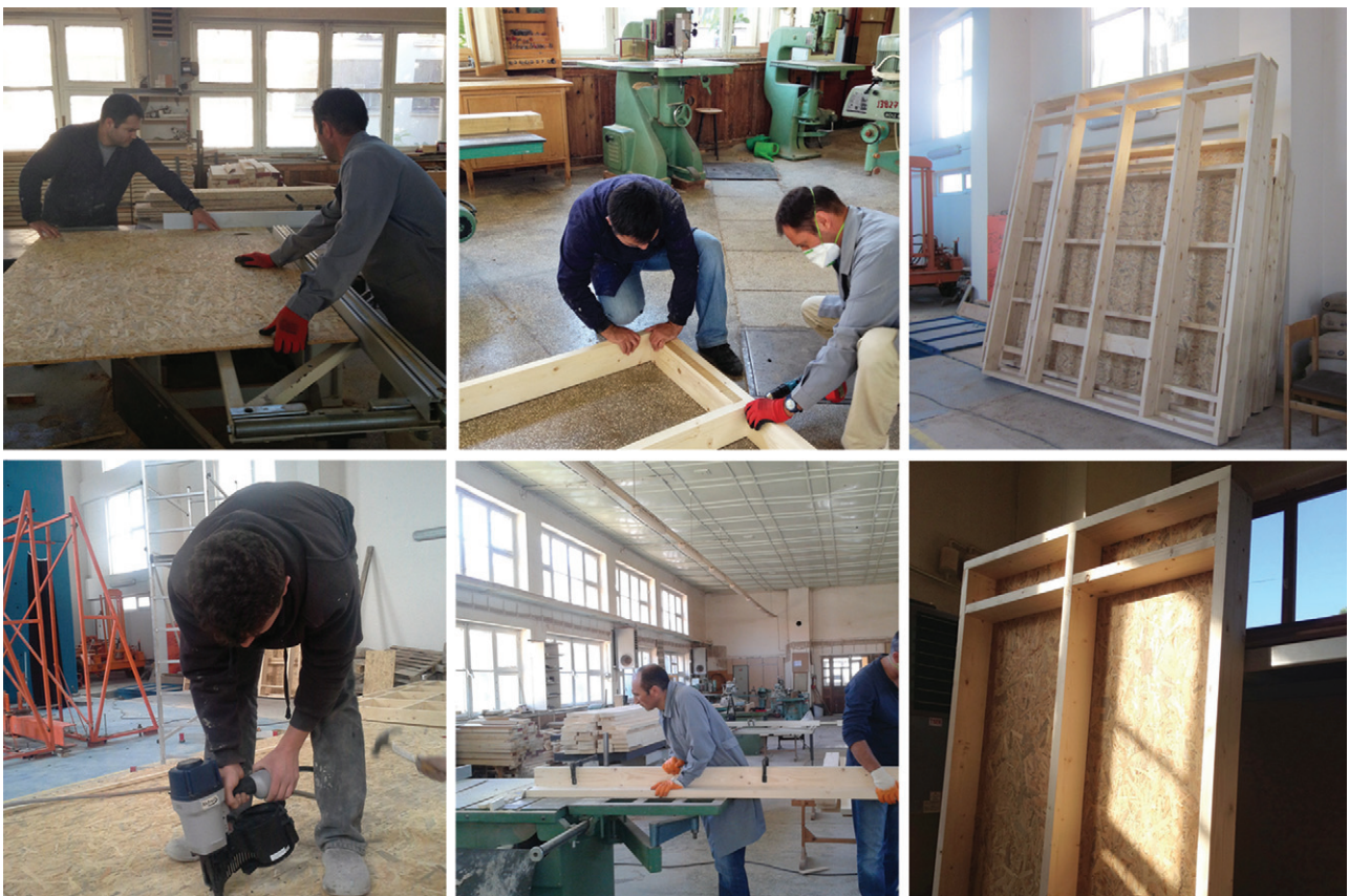
Figure 2. Manufacturing process of test specimens
