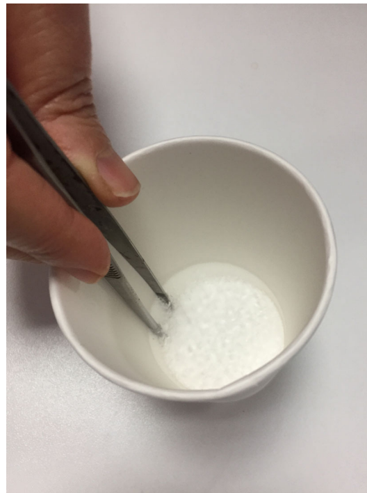
FIGURE 2 Cooling the tip of the forceps in liquid nitrogen which was transferred to the cardboard cup
