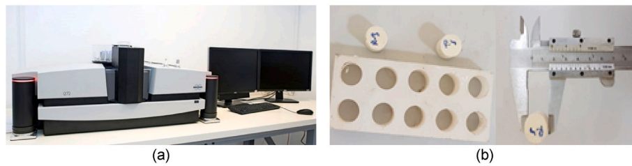
Fig. 7. (a) Computed tomography device, (b) test specimens ( \text{Ø}18 \times 20 \text{ mm} ).
