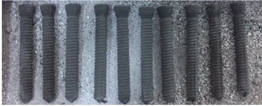
Fig. 10 – The green part of thermal debinding.
