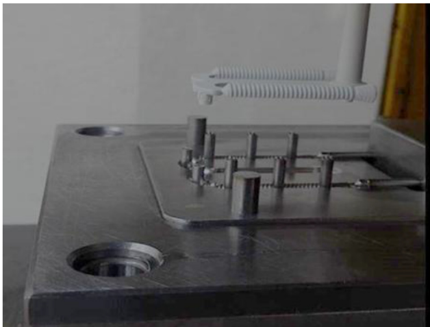
Fig. 5 – Green part production with 60% feedstock by volume.
