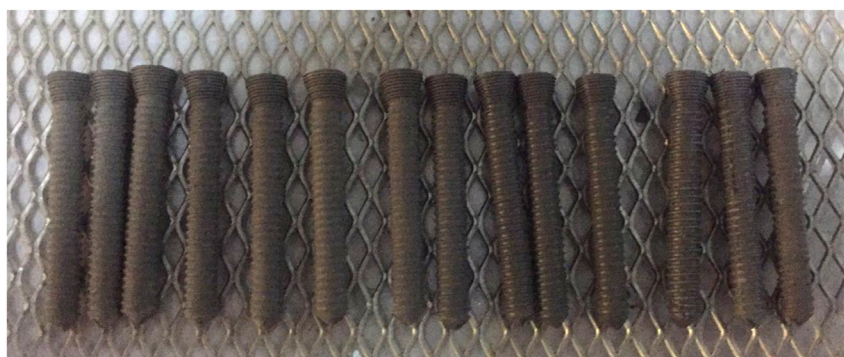
Fig. 9 – The Green part solvent debinding.
