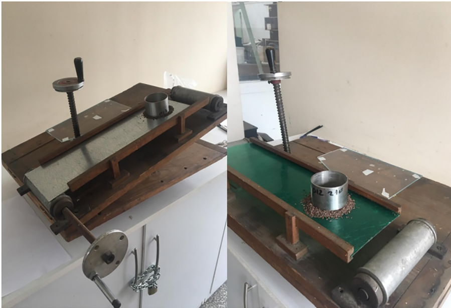
FIGURE 3 Determination of static friction angle with galvanized and PVC surfaces
