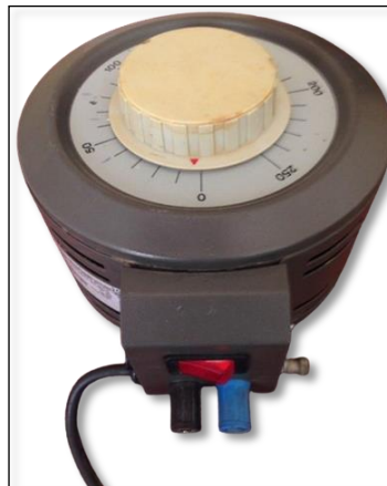
Figure 3.11: Voltage Regulator Device.
