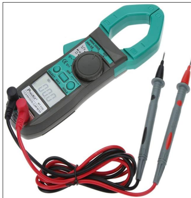
Figure 3.13: Multi-meter device for voltage and current readings.
