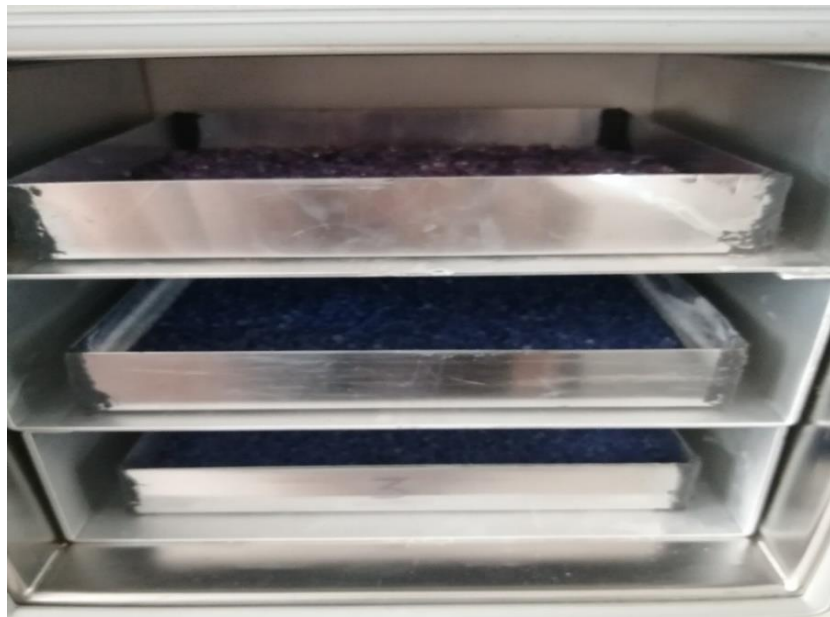
Figure 3.20. Drying process of SiO 2
