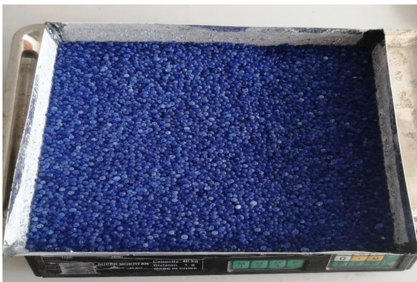
Figure 3.22. Silica gel after the drying process
