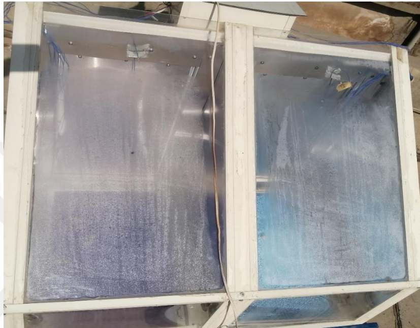
Figure 3.28. water droplets condensed on the cover surface
