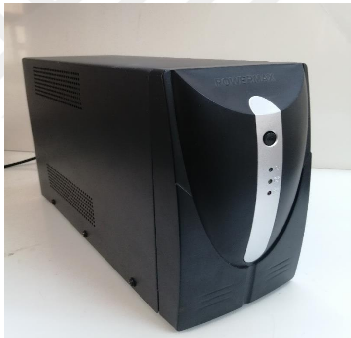
Figure 3.12. UPS power supply
